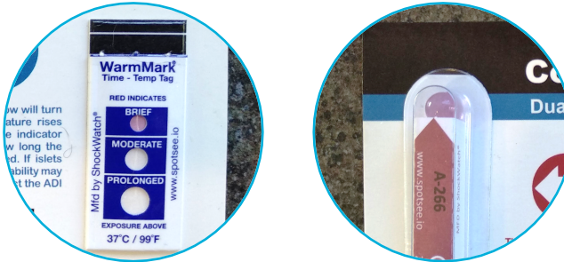
A temperature monitor showing the cold (left) and warm (right) temperature triggers.
