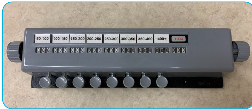
A nine-channel benchtop cell counter is used to facilitate counting.
